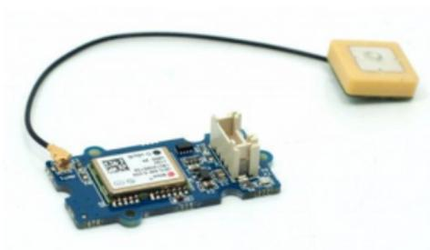
Figure 7- Module GPS
