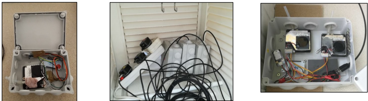
Figure 4: detail of one initial SDS011 sensor box (left), three of them in the meteorological shelter at «Laënnec» (center), New experimental package with two associated sensors are (right) to be able to evaluate some bias.
