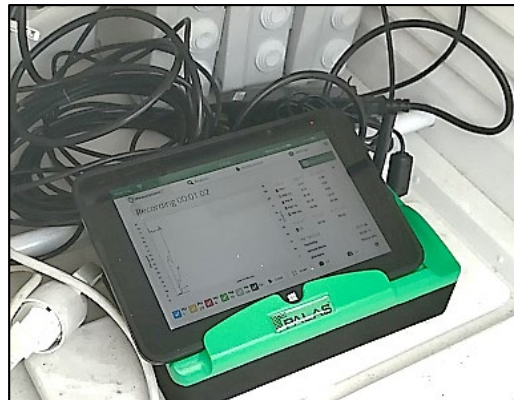
Figure 7: The FIDAS Frog was placed in the meteorological shelter at «Laënnec».
